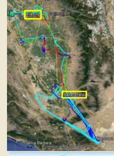
Composite Flight Track Map showing repeated spirals at each of the six waypoints, highlighting Fresno and Bakersfield, the focus for this study
